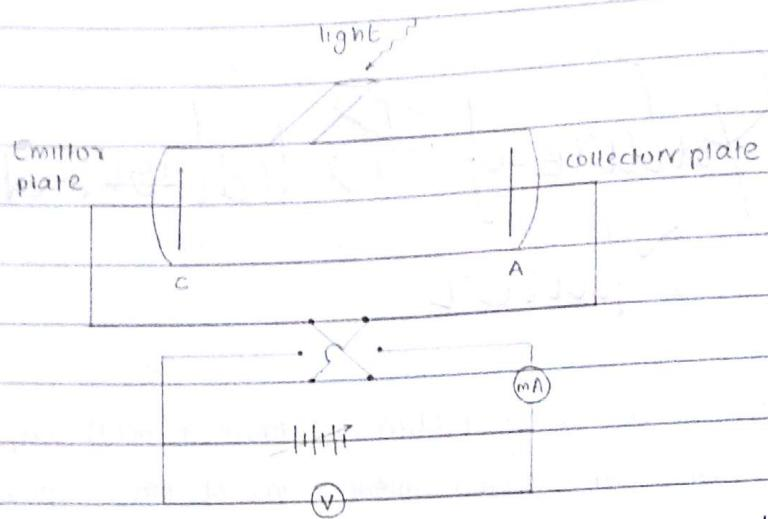
It consists of two metallic plates C and A, arranged in a evacuated chamber. The plates are connected to a source of voltage through a commutator so that the potentials can be adjusted. There is an opening at the top of the tube. Light is allowed to fall on the plate C through a transparent window arranged at the top of the tube. Then photoelectric emission takes place and current begins to flow through the circuit and this current is known as photoelectric current.
