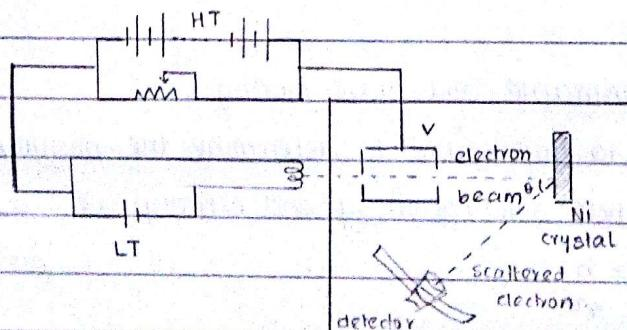
The experimental setup consists of an electron gun connected to a low tension source. The gun emits an e-beam and is allowed to fall on Ni crystal through a cylinder which is connected to a high tension source. The voltage across the cylinder is adjustable.
